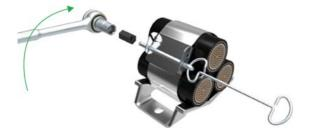
Pull slack into outer loop. Insert split pin from right hand side around outer layer of strap about 10mm from end. Push plastic shear torque adaptor fully onto the end of the split pin and attach 13mm socket wrench. To tension the strap rotate key anti-clockwise with the socket wrench until the adaptor shears.
