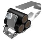
Fasten base to support with M10 fixings. Loop strap through base and around cables. Standard duty = 2 loops. Heavy Duty = 3 loops.
