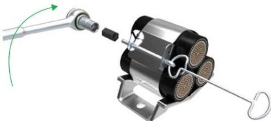
Pull slack into outer loop. Insert split pin from right hand side around outer layer of strap about 10mm from end. Push plastic shear torque adaptor fully onto the end of the split pin and attach 13mm socket wrench. To tension the strap rotate key anti-clockwise with the socket wrench until the adaptor shears.
