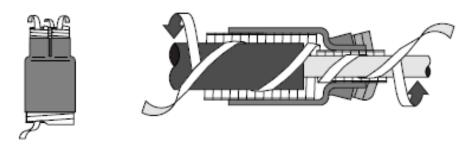
2. After measuring required length, install RJS – Series silicone rubber phase re-jacketing sleeves.
