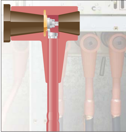
T-adapter for perpendicular connection of the termination to SF 6 -insulated switchgear
