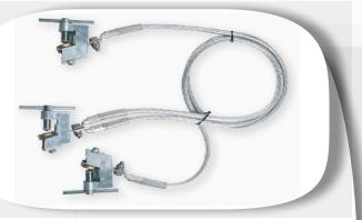
Short Circuiting Straps are used to short the positive and negative circuit of a D.C Feeder section. Each Strap consists of three J117-NSE clamps fitted with flexible Copper leads.
