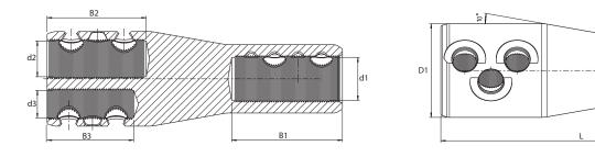
Mechanical cable lug > Connects conductors of different cross sections and conductor materials
