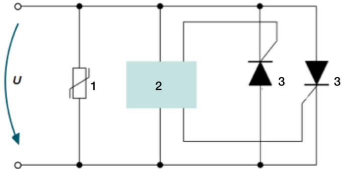
**Equivalent circuit of voltage limiting device**
