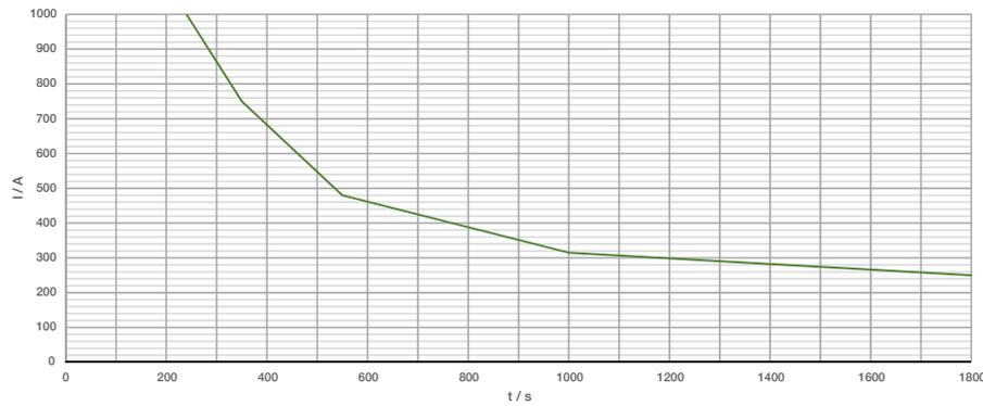
Maximum current versus time, reversible. The temperature rise at these load conditions is much more than 75K.
