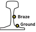
1. Clean the brazing & grounding area with a grinding machine (special pin required).
