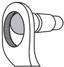
3. Pull the trigger. The pin lifts and creates an arc. The special flux powder cleans and prepares the surface.
