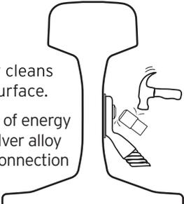
5. Finish by knocking off the control shaft of the brazing pin with a hammer. You have now created an extremely efficient and reliable silver connection.
