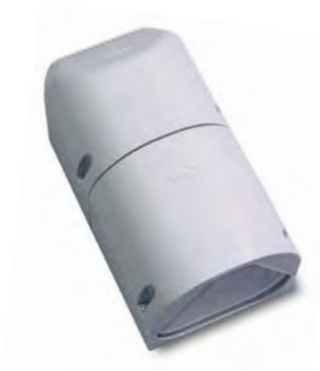
NEC Extension Trough, 3 entry Created by coupling NEA trough to NEB Terminals can be installed in either upper chamber (NEA) or lower chamber (NEB) Height 180mm, Width 98mm, Depth 93mm
