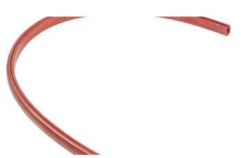
nVent RAYCHEM G-02 is a silicone grommet that protects the heating cable at sharp edges such as endplates of insulation cladding, flanges, etc. It can be cut-to-length and resists temperatures up to 215  $^{\circ}$ C.
