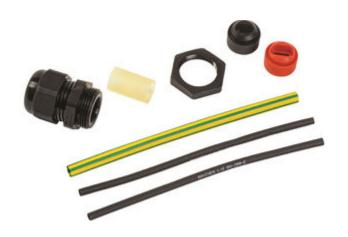
nVent RAYCHEM C25-21 is a hot-applied connection kit for terminating all nVent RAYCHEM self-regulating and power-limiting industrial parallel heating cables to a junction box.
