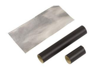
These end seal kits are designed for the termination of nVent RAYCHEM industrial heating cables. The end seal kit employs easy to use heat-shrinkable tubing with an adhesive, that when heated forms a semi-flexible moisture proof encapsulation. Due to the low profile design the finished termination can be installed directly on the pipe. One end seal kit is required for each termination.
