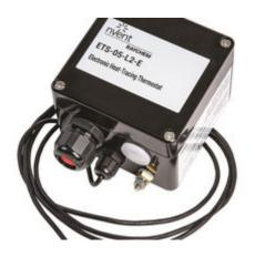
nVent RAYCHEM ETS-05 hazardous area electronic surface sensing thermostats provide accurate temperature control for heating cables. ETS-05-L is adjustable to 199 °C, ETS-05-H up to 499 °C. ETS-05 has a LED to indicate status of the thermostat, heating cable and sensor.
