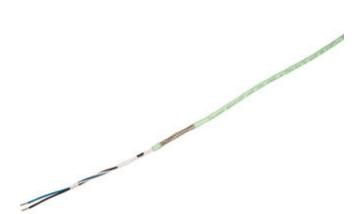
nVent RAYCHEM FHT constant wattage parallel trace heating cables provide freeze protection and process temperature maintenance, up to 230 °C. They can withstand routine steam purges and intermittent exposure to 260 °C, available in 230 and 400 V and approved for use in hazardous areas. The fluoropolymer outer jacket (-CT) provides high chemical resistance against aggressive organics and corrosives.
