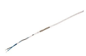
nVent RAYCHEM FMT constant wattage parallel trace heating cables provide freeze protection and process temperature maintenance, up to 150 °C. They can withstand routine steam purges and intermittent exposure to 200 °C, 230 V supply and FEP outer jacket. Approved for use in hazardous areas.
