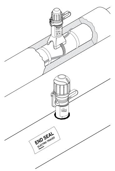
Both the nVent RAYCHEM E-100-E and E-100-L-E are accessible, re-entrable end seals, the E-100-E without a light, the E-100-L-E with a signal light. Both end seals can be used with all nVent RAYCHEM BTV, QTVR, XTV, KTV or VPL industrial parallel heating cables. They are approved for use in hazardous areas. They are extremely rugged - made of a strong, moulded part with 4 mm wall thickness.
