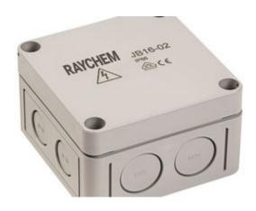
nVent RAYCHEM JB16-02 and JB-82 temperature-resistant polycarbonate junction boxes for non-hazardous areas. For use with nVent RAYCHEM self-regulating heating cables, to make a power connection, tee, splice, powered splice/tee. Up to four heating cables, or three heating cables and the appropriate size power cable can be connected through the four entries and connected to the rail mounted terminals.
