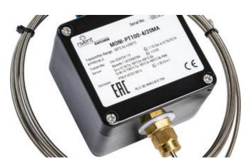
nVent RAYCHEM MONI-PT100-4/20MA is a PT100 sensor connected to a 4-20 mA transmitter built into a black glass fiber reinforced polyester junction box. Suitable for hazardous areas.
