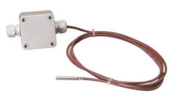
nVent RAYCHEM MONI-PT100-NH sensor is a two-wire platinum resistance temperature detector (RTD), supplied with glass fiber reinforced polycarbonate junction box, for non-hazardous areas.
