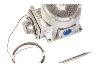
nVent RAYCHEM Raystat-EX-02 is a hazardous area mechanical surface sensing thermostat providing temperature control for heating cables. Switching temperature range -4 °C to 163 °C, adjustable externally to the Ex enclosure by a dial mounted under a bolted-on cover and seal. Switching current capacity is 22 A.
