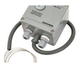
nVent RAYCHEM T-M-10-S/+x+y is a non-hazardous area mechanical surface sensing thermostat providing temperature control for heating cables. Available in ranges: 0 °C-50 °C; 0 °C-200 °C; 50 °C-300 °C. The temperature set point can be adjusted without opening the enclosure via a removable plug in the lid. Direct connection of the heating cable is possible, switching current capacity is 16 A.
