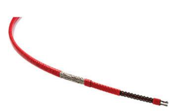
nVent RAYCHEM XTV self-regulating trace heating cables are mainly used for freeze protection of pipes and vessels that require steam cleaning and process temperature maintenance, up to 250 °F/121 °C. They withstand intermittent exposure to 482 °F/250 °C. The fluoropolymer outer jacket (-CT) provides high chemical resistance against aggressive organics and corrosives.
