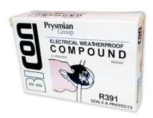
Electrical connections may be protected from moisture and corrosive vapours by use of a non-hardening waterproof sealant (R391/392) supplied by Prysmian. The material has the consistency of putty, has good insulating properties and can be moulded around terminals and connectors providing a moisture and mechanical seal for any form of enclosure.
